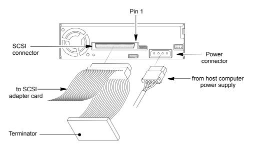
**Figure 2-4** Connecting a SCSI cable (tape drive is last device on the bus)
